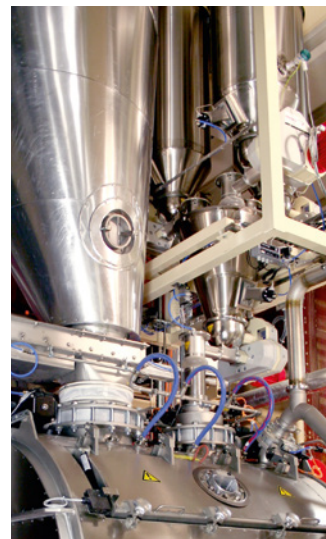
Coperion K-Tron screw feeders in a vacuum coating process
